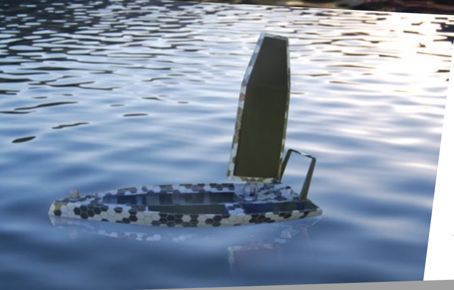
Man-O-War SSUOV with SolarSail™ stowed on deck
